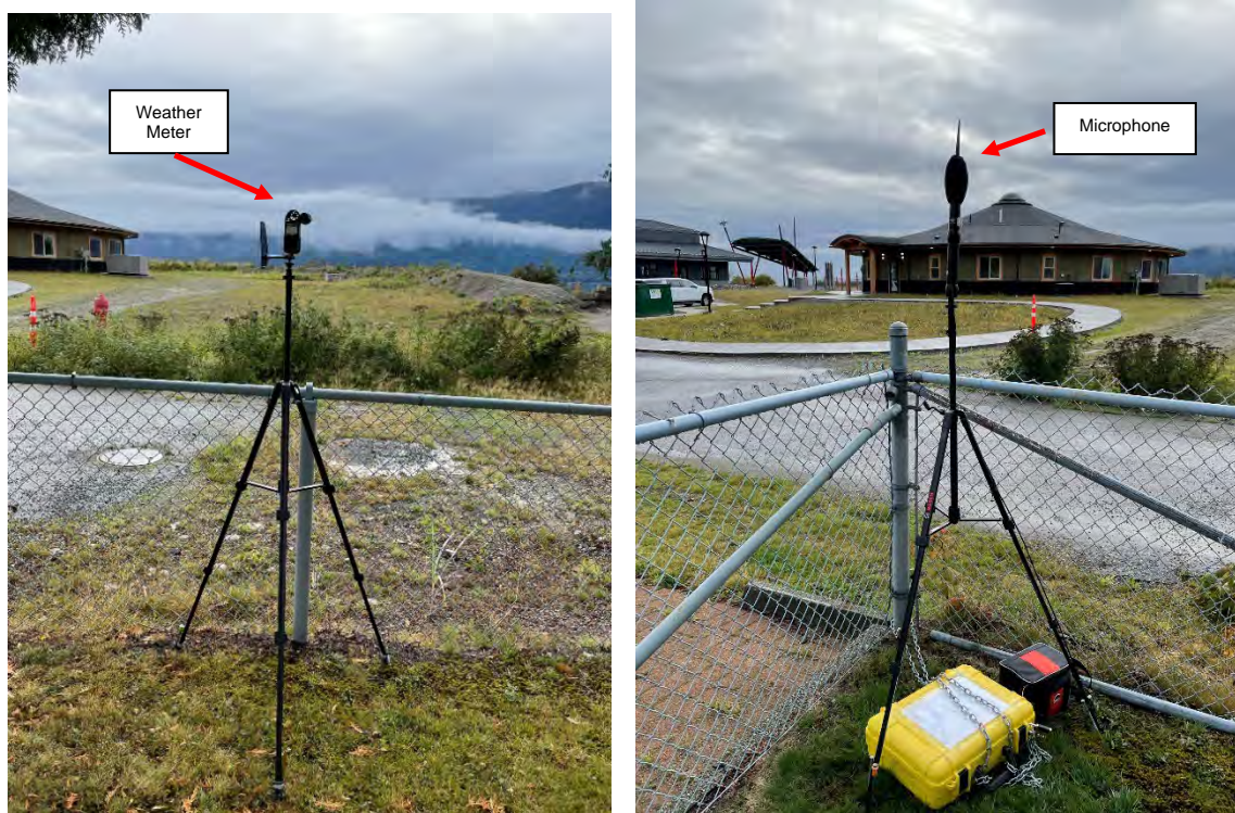
Photo 3 Sound Level Meter and Weather Meter Setup at BL3
