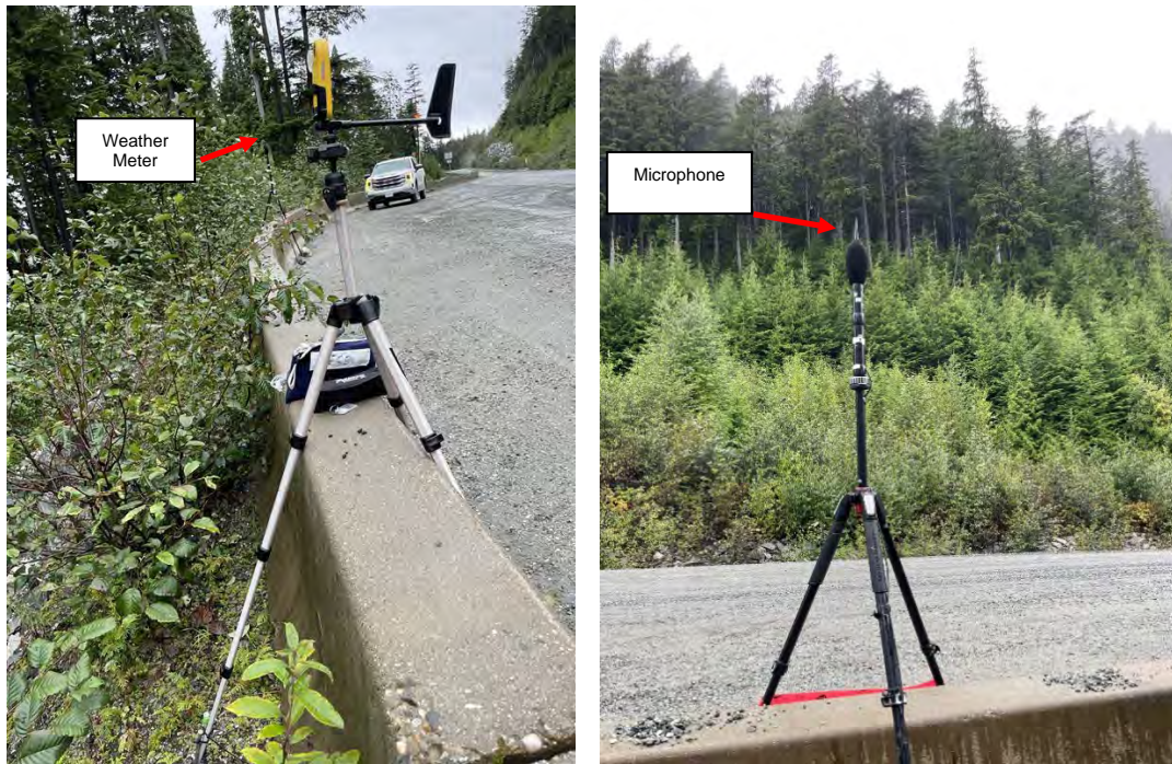
Photo 2 Sound Level Meter and Weather Meter Setup at BL2
