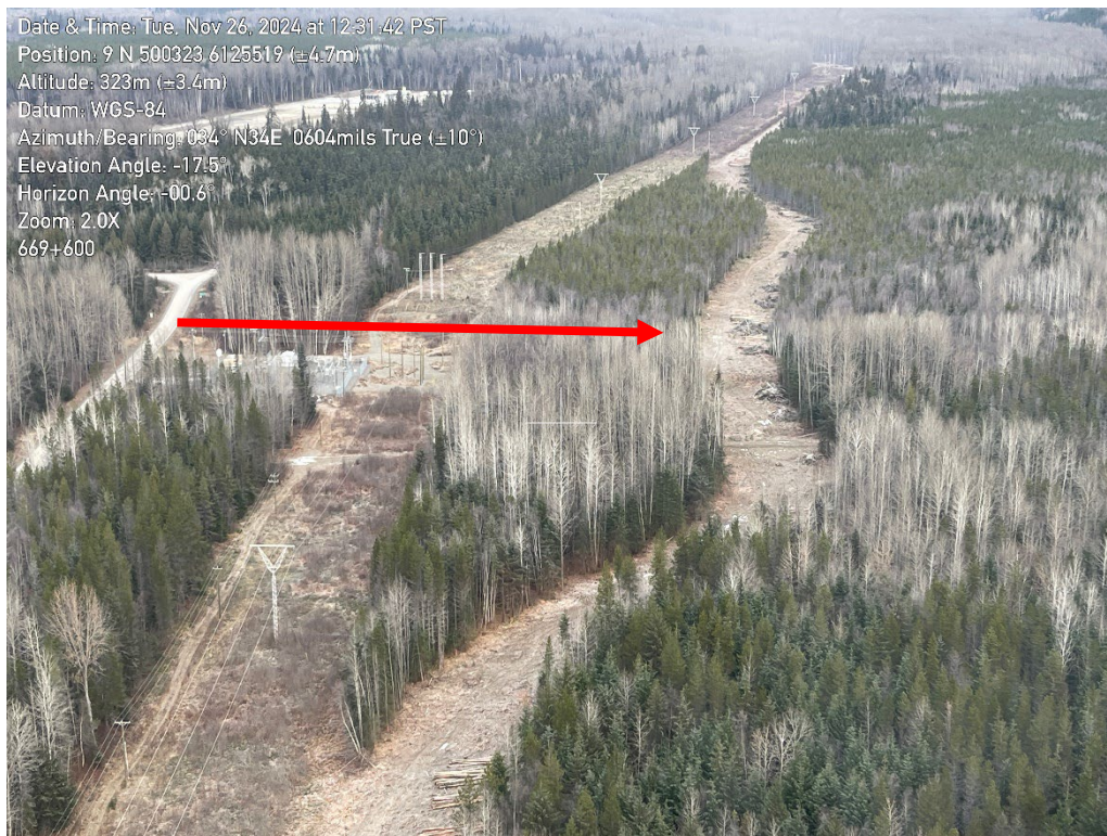
Photo 3. Cleared pipeline ROW at KP 668+600, where it temporarily diverges from an existing, non-Project transmission line ROW. Road #8 from Nass Road across the transmission line ROW to the Project ROW indicated in red.
