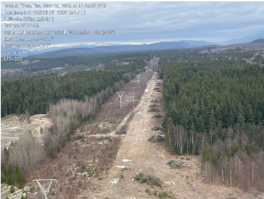
Photo 5. Cleared pipeline ROW at KP 676+400 adjacent to existing, non-Project transmission line ROW.
