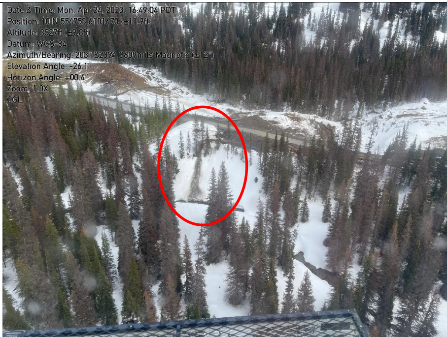
Photo 9. KP 144+650 evidence of filter bag discharge reaching Environmentally Sensitive Receptor (watercourse).
