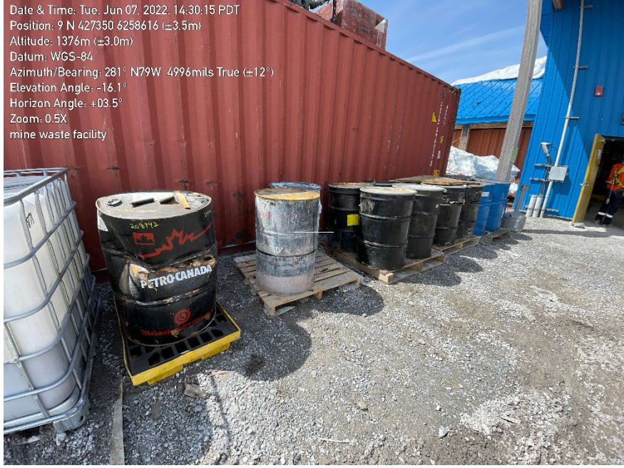
Photo 5. Waste oil stored at Mine Site Waste Transfer Area without secondary containment.
