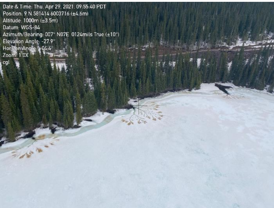
Photo 27. KP587+450 (approximate). Sediment from RoW entering lake.
