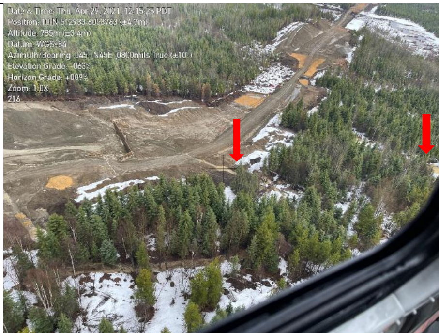
Photo 12. Sediment laden water into S4 at KP 216+100, which then reaches S3 at KP 215+700.
