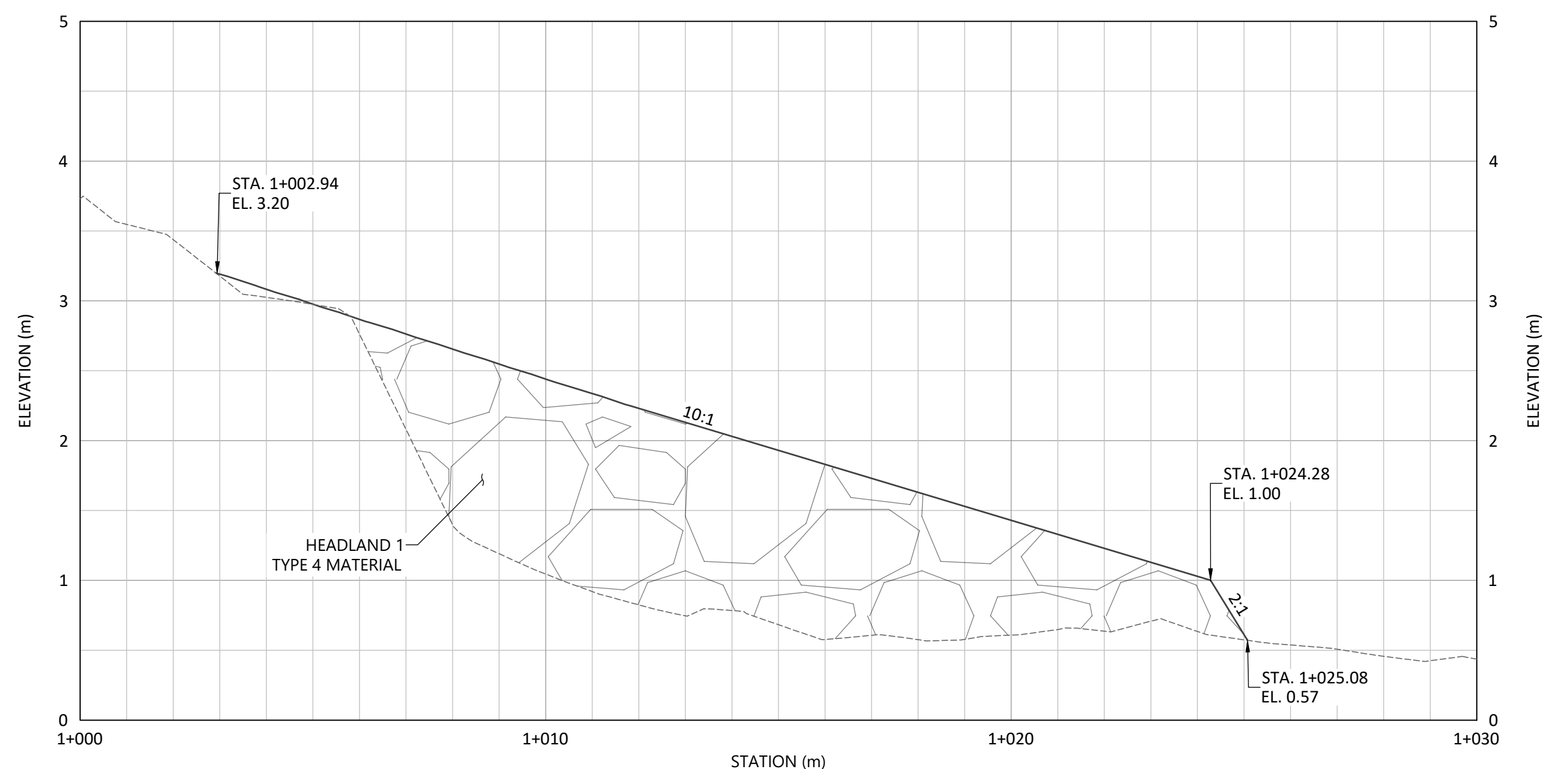
PROFILE - HEADLAND 1 CENTERLINE SCALE 1:100 | 3x VERTICAL EXAGGERATION
